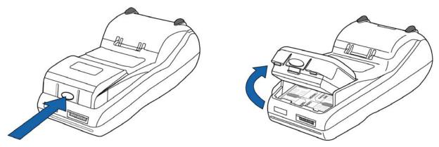
Figure 18 **Detaching the Smart Battery from the V<sup>x</sup>670 Terminal**
